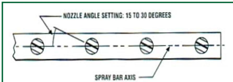
Set the spray bar nozzles at an angle between 15° and 30°.
